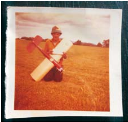
1970s Quarter Midget pylon racer. Cassutt with Supertigre 2.5cc engine
